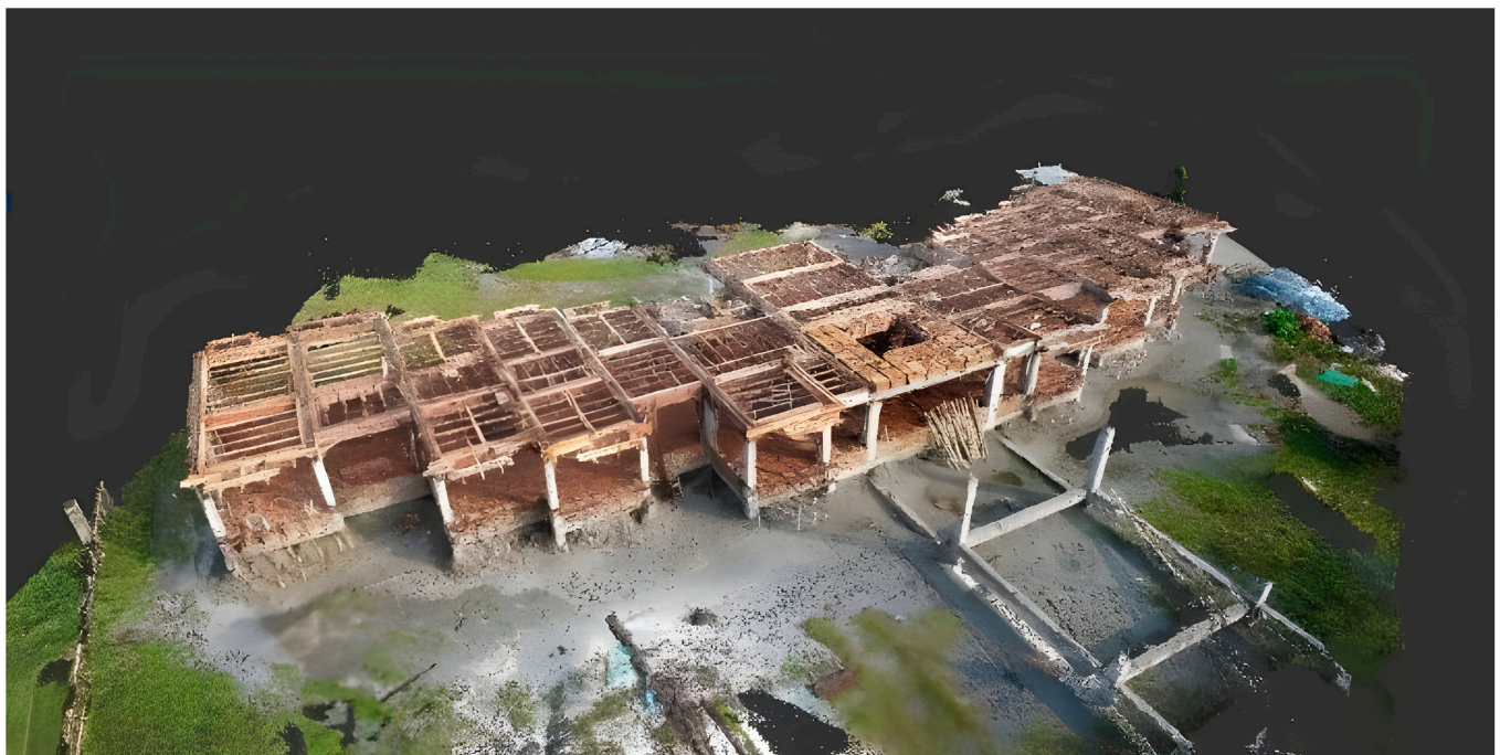
Fig. 11. Generation of point cloud and 3D texture mesh.
